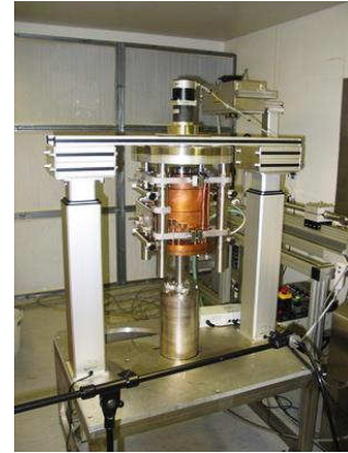
Figure 1: Set-up for RF-Photo Guns.
