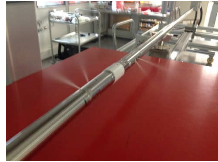
Figure 4: Two coupled lances with 4 nozzles.
